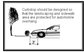
required for all head-in parking spaces adjacent to landscaped areas. Wheel stops shall be designed so that the overhang of vehicles is contained totally within the parking space. When wheel guards are used, they shall be centered 3 feet from the property line for 90 degree parking, 2.3 feet for 60 degree parking, and 2.0 feet for 45 degree and 30 degree parking.
