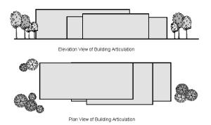
b. Vertical Articulation: No horizontal wall shall extend for a distance over one hundred (100') feet without changing height by a minimum of three (3') feet.
